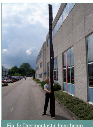
Fig. 5: Thermoplastic floor beam
