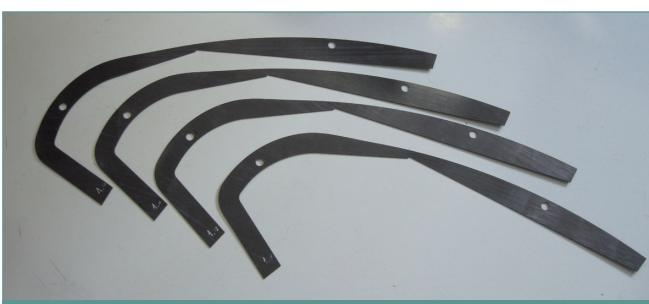
Fig. 13: Flat rib preforms
