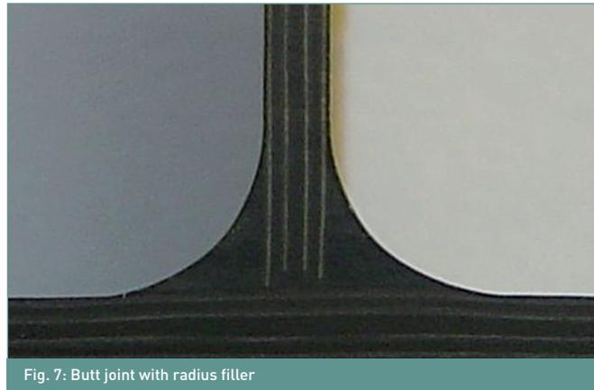
Fig. 7: Butt joint with radius filler
