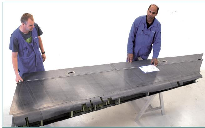
Fig. 3: Welded Gulfstream G650 thermoplastic rudder
