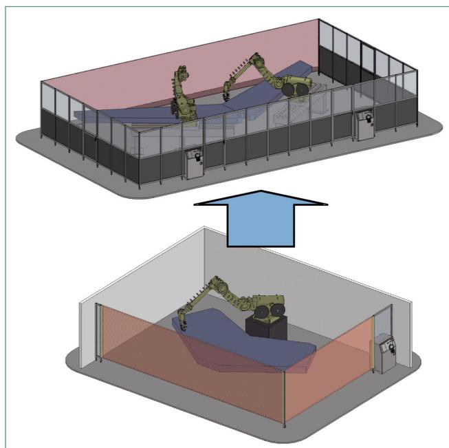
Fig. 16: Fibre placement R&D cell and production cell
