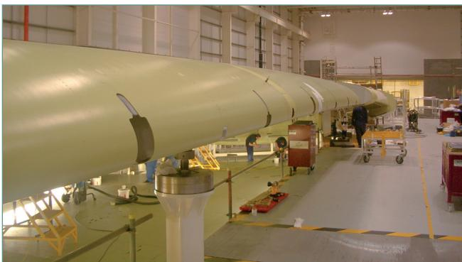
Fig. 1: Welded fixed wing leading edge on an A380 wing (photo courtesy Airbus)
