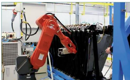
Fig. 4: Induction welding of Gulfstream G650 rudder and elevators
