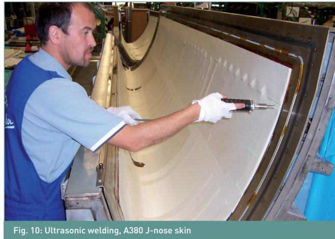
Fig. 10: Ultrasonic welding, A380 J-nose skin
