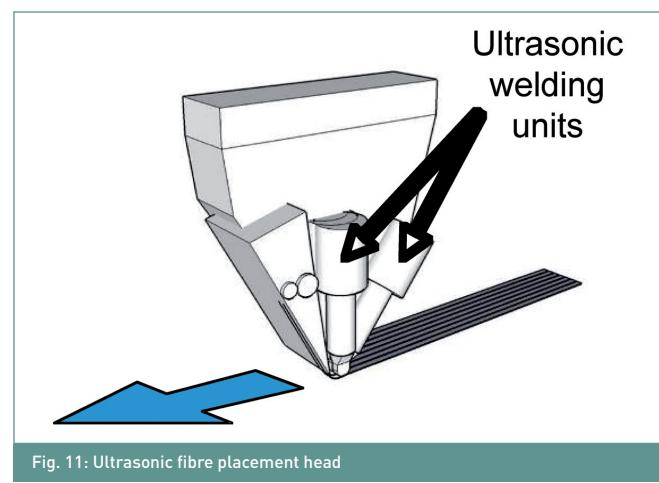
Fig. 11: Ultrasonic fibre placement head
