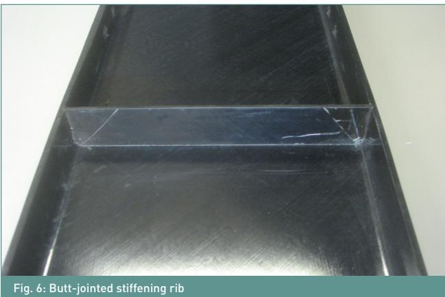
Fig. 6: Butt-jointed stiffening rib
