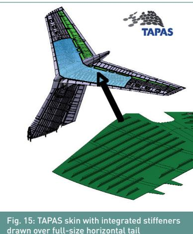
Fig. 15: TAPAS skin with integrated stiffeners drawn over full-size horizontal tail
