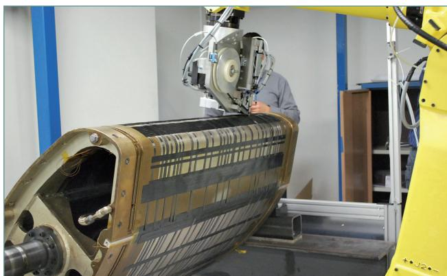
Fig. 12: Butt jointed sine wave beam
