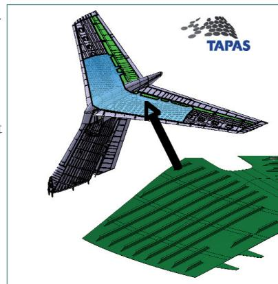
Fig. 15: TAPAS skin with integrated stiffeners drawn over full-size horizontal tail
