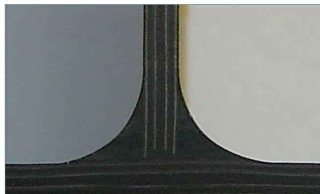
Fig. 7: Butt joint with radius filler
