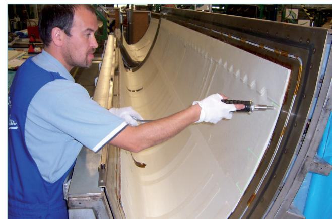
Fig. 10: Ultrasonic welding, A380 J-nose skin
