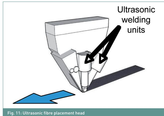
Fig. 11: Ultrasonic fibre placement head
