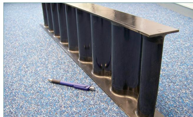
Fig. 8: Butt jointed sine wave beam
