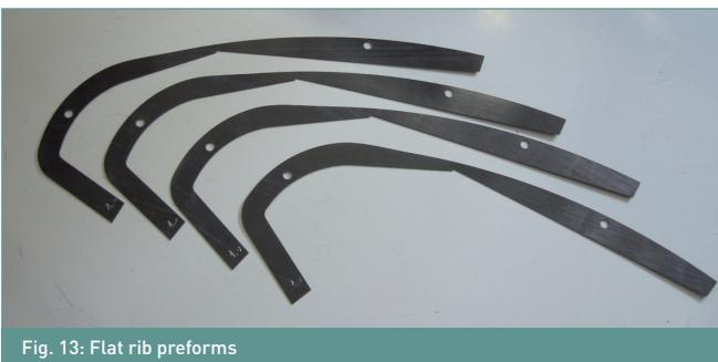
Fig. 13: Flat rib preforms
