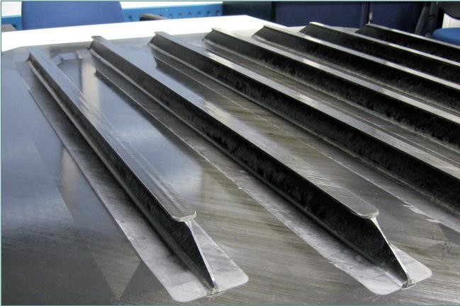
Fig. 9: Skin panel with integral butt joined T-stringers
