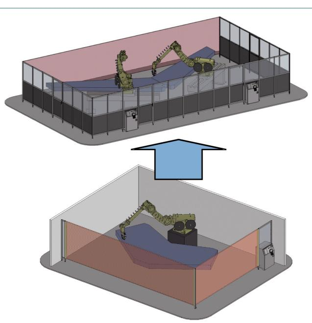
Fig. 16: Fibre placement R&amp;D cell and production cell
