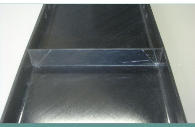
Fig. 6: Butt-jointed stiffening rib
