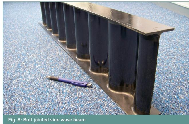
Fig. 8: Butt jointed sine wave beam
