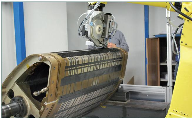
Fig. 12: Butt jointed sine wave beam
