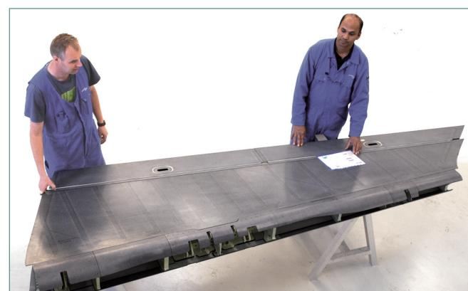
Fig. 3: Welded Gulfstream G650 thermoplastic rudder
